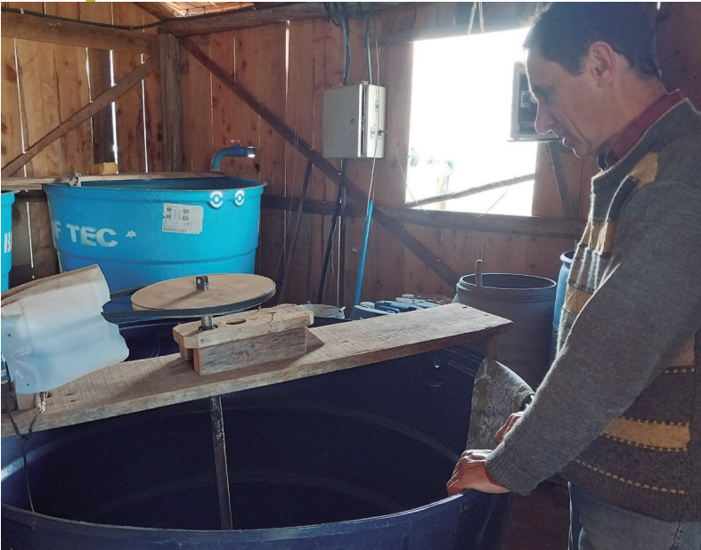
Aerator with washing machine motor, in a water tank, to reproduce communities of microorganisms, on the Marcos Mosquer site, 2025
