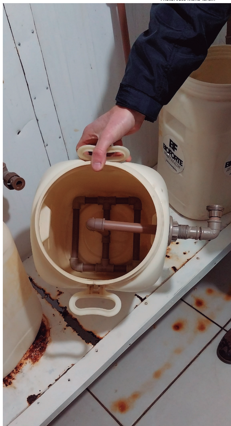
Bioreactor with aerator at the bottom. Mãos na Terra [Hands on Earth] Group 5 , 2025
