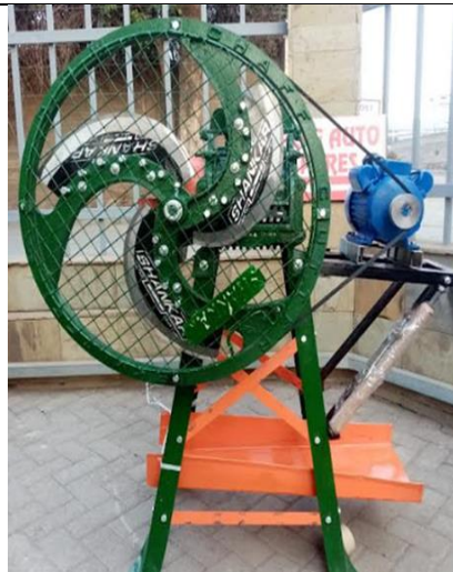
Figure 13: Motor-driven chaff cutter
