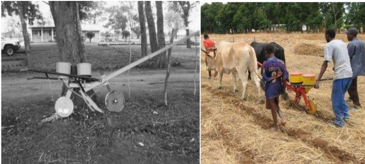
Figure 6: Animal traction direct planter cutting through mulch
