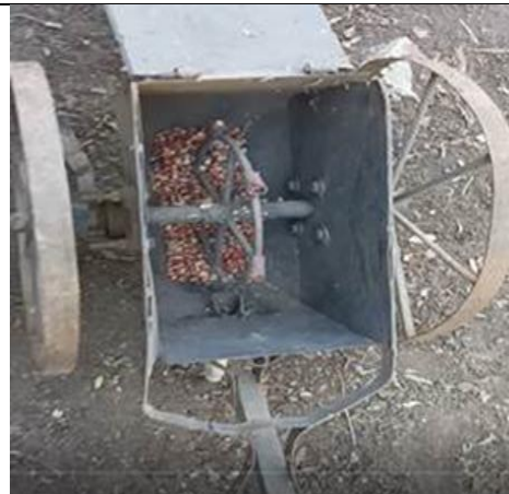
Figure 8: Picture showing the seed compartment of the metallic manual hand-driven seed planter
