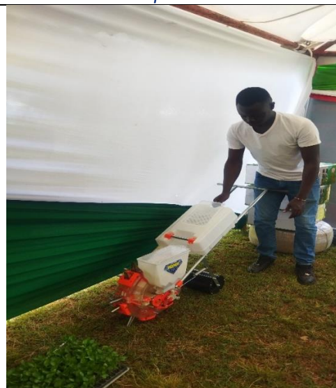
Figure 10: Manual hand-driven seed planter with fertilizer compartment fabricated by FineTouch Africa (@ Ksh. 24,000)
