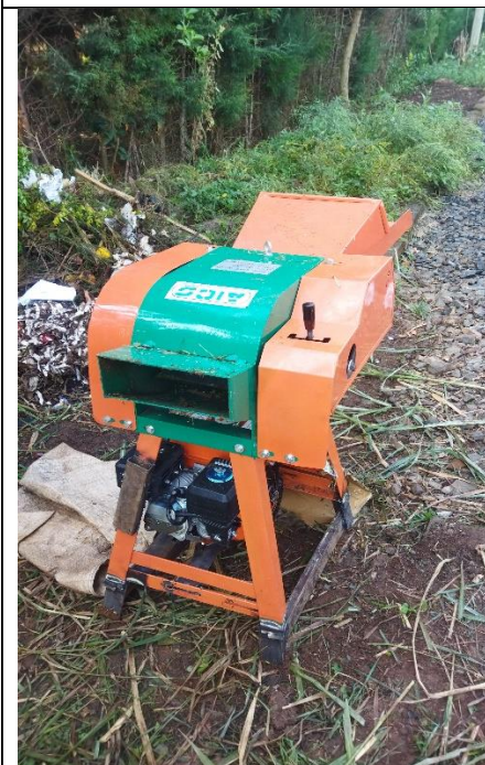
Figure 15: Motor-driven chaff cutter seen at Eldo Fabricators
